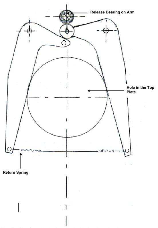
Move Top Plate forward or back so that the Iris Arms <u>just</u> clear the hole to allow the clay to fall through. <u>DO NOT</u> over adjust! This will cause excessive movement of the Iris Arms and damage the mechanism. Lock in place when set up is correct.
