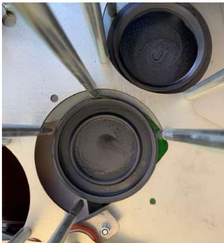
Carousel showing reversed targets which can be placed alternately in each stack, if required.
