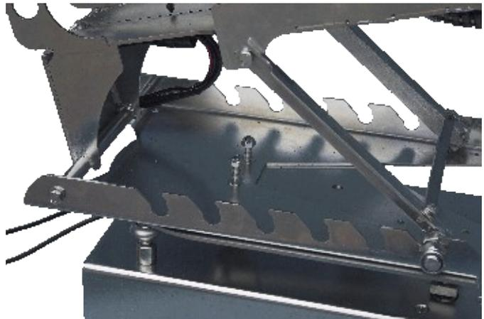
base of the trap, refit the washers and securely tighten the nuts to hold the trap to the turner plate. Once the trap is secured to the Oscillating base, plug the three-pin plug, from the base, into the socket on the trap. The controller is then plugged into the socket on the Oscillating base.
