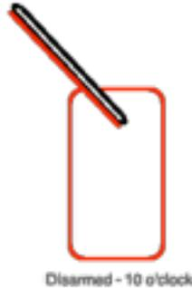
In this position, the trap is safe and there is no risk of the trap firing by accident, however the spring is still under some tension.
