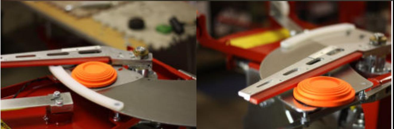
Once this clearance has been achieved across the entire plate, lock the plate setting by tightening the lowermost serrated nuts. Once locked, you should never have to adjust these nuts again.
